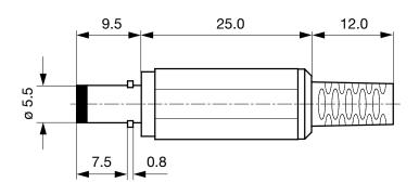
Cable diameter max. 4.0 mm
