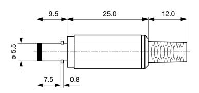
Cable diameter max. 4.0 mm
