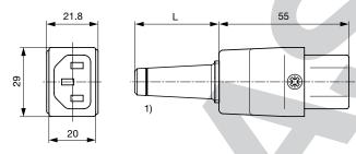
1) Cut cable guard to suit cable diameter
