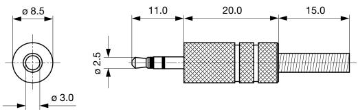
Cable diameter max. 3.0 mm
