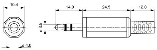
Cable diameter max. 4.0 mm
