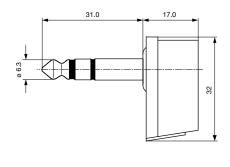
Cable diameter max. 8.0 mm
