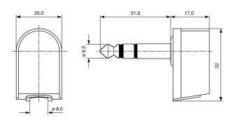
Cable diameter max. 8.0 mm
