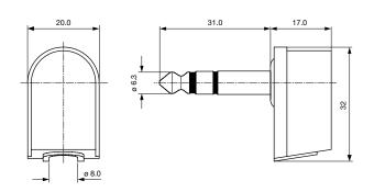
Cable diameter max. 8.0 mm
