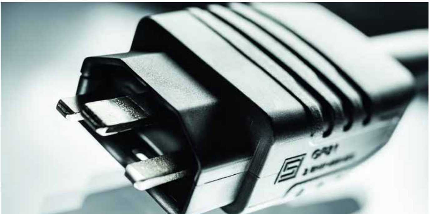
SCHURTER GP21: 400VDC power plug according to IEC TS 62735-1 for systems up to 2.6 kW
