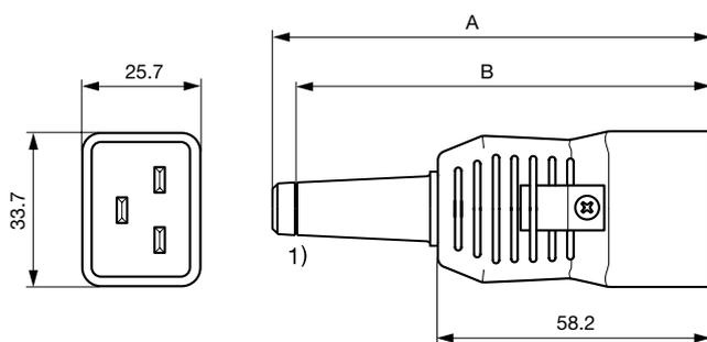
1) Cut strain relief 8 (10) mm here for 10 mm cable
