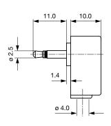
Cable diameter max. 4.0 mm
