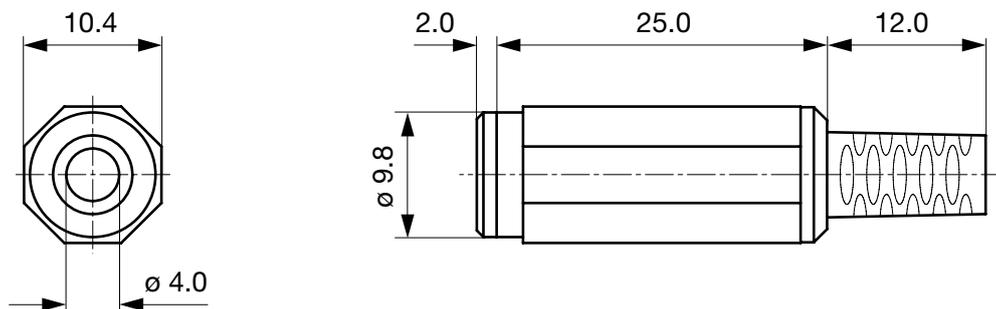
Cable diameter max. 4.0 mm
