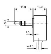
Cable diameter max. 4.0 mm
