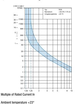
Tripping Characteristics thermal In  $\geq 3 \dots \leq 15 \text{ A}$
